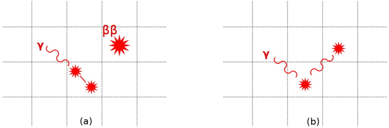
Figure 4.1: Illustration of the SS (a) and MS (b) event topologies for a gamma( \gamma ) and aa double-beta ( \beta\beta ) decay event, projected onto wire grid.
