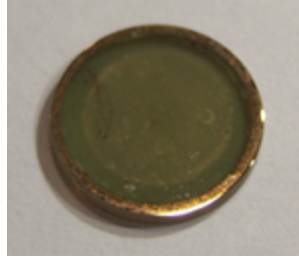
Figure 6.3: Picture of a photocathode. It is a 1mm sapphire disk on which gold was evaporated to a thickness of 22 nm. Between the gold and the sapphire is a layer of chromium to facilitate adhesion. The discoloration on the edge is a result of the phosphor bronze plate contact for HV biasing.
