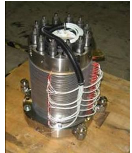
Proton PEM cell stack for UK Vanguard subs
