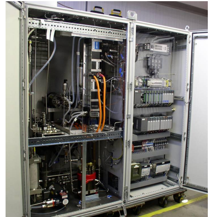
2 kW closed loop DRFC on test 400 psig H 2 / 375 psig O 2
